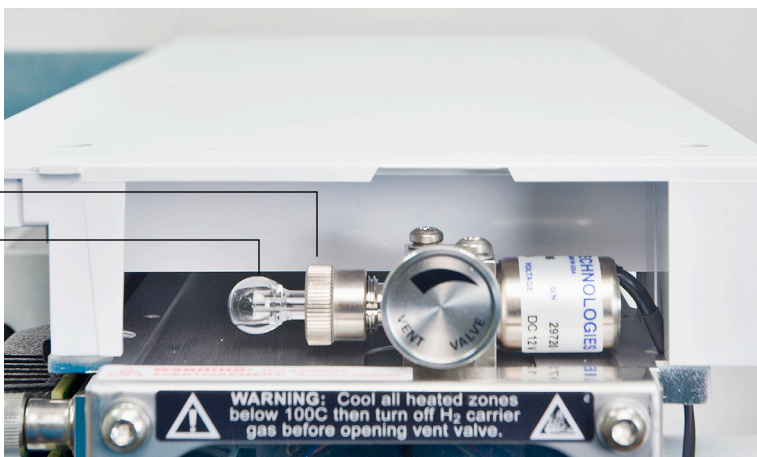
Figure 15 Removing the EI calibration vial
